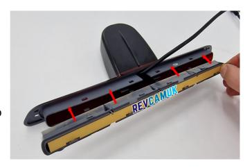
Take note of the photo showing where the wire exits the camera. There is a cut out to avoid the cable being pinched.
